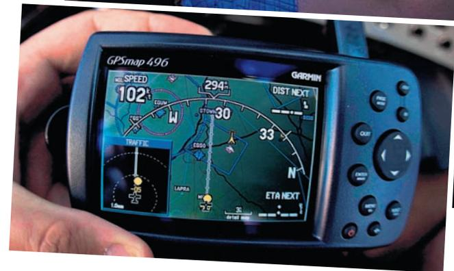
CAP-10, and to ensure that we could verify the traffic information displayed by the unit we flew in company with an RV-6A. We used GPS-measured distances along a common course line to check the accuracy of the range information.
